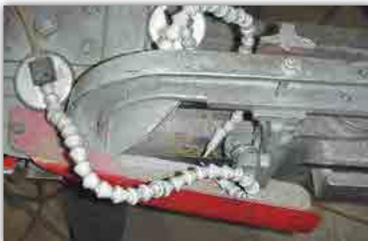
Minimum quantity lubrication used on a horizontal saw
