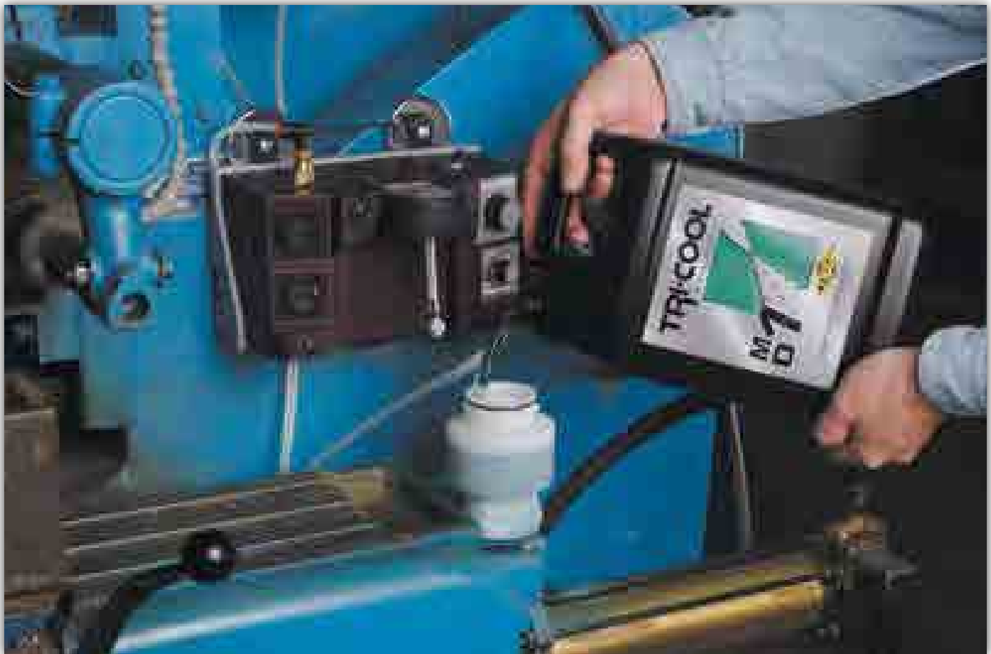
Micro-dispenser being filled with Tri-Cool MD-1 lubricant
