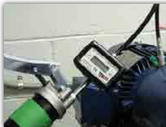
Grease meter being used with Spectrum Grease Identification Products to ensure the right grease goes into the right piece of equipment.
